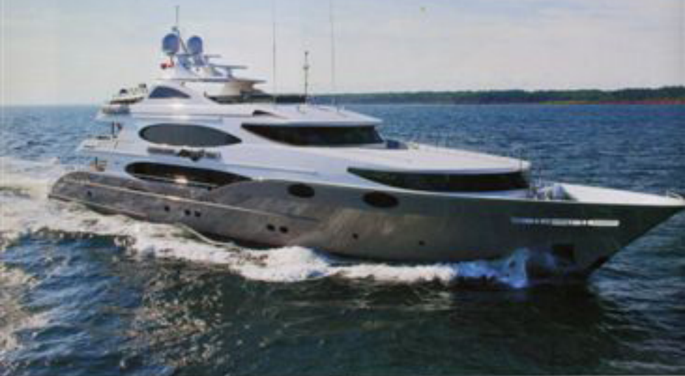
She is a tri-deck with a beam of 28 ft. (8.6m) and an aluminum semi-displacement hull and aluminum superstructure. The propulsion system from two Caterpillar engines 3512E, producing 2200hp. This provides a top speed of approximately 20 knots. She has a cruising range of 3000 nautical miles at 10 knots. The Destination FORTHABER 100 has an advanced stabilizing system featuring Quantum 2s active fin with digital controls with Zero Speed™. The yacht has a Quantum 150hp bow thruster.
