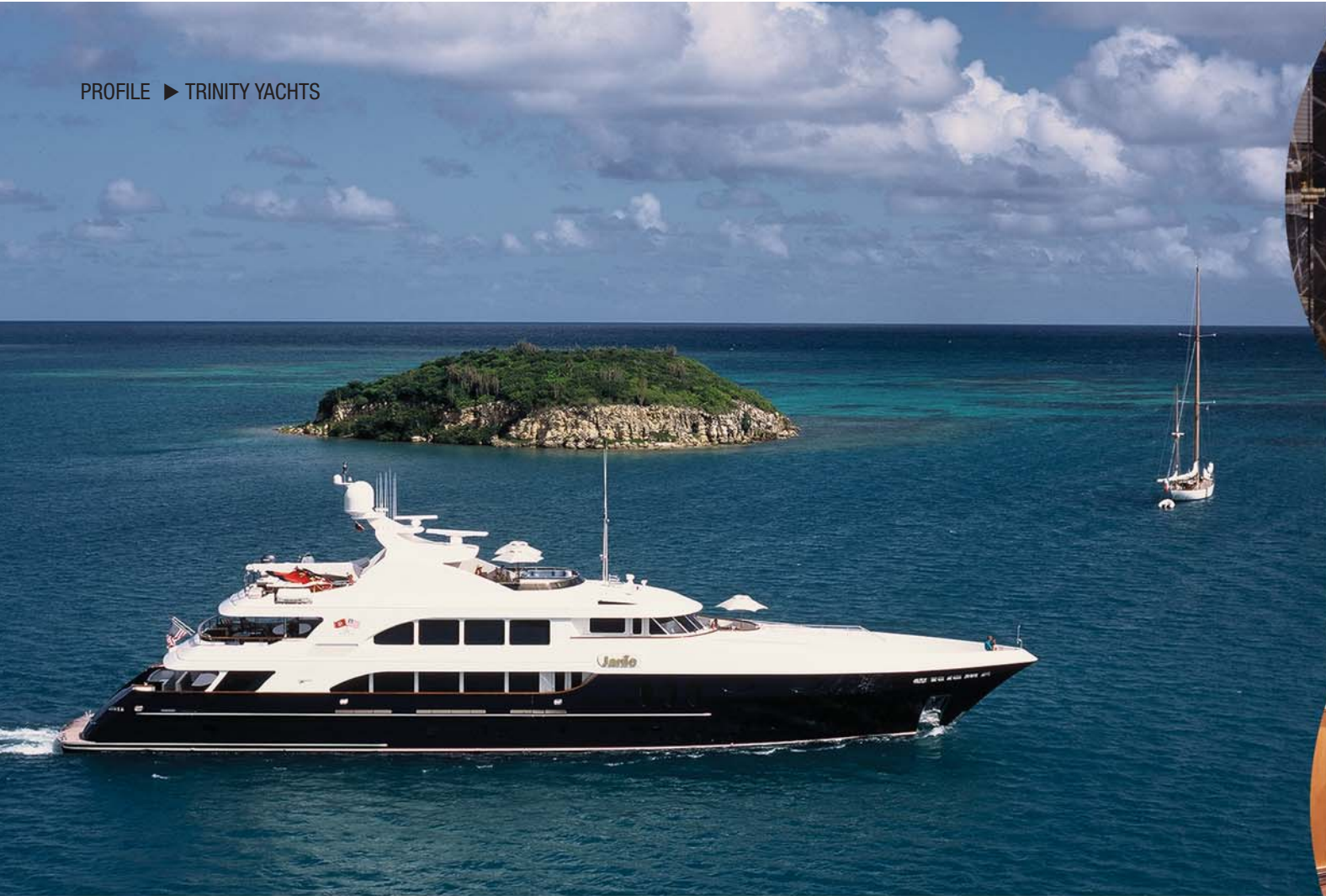
Pictured above: The 157 ft. (47.9m) M/Y JANIE is capable of cruising at 18.5 knots. Its draft of 7 ft. 1 inch (2.16m) will allow it to navigate many areas of the Bahamas while maintaining her transatlantic capability;
